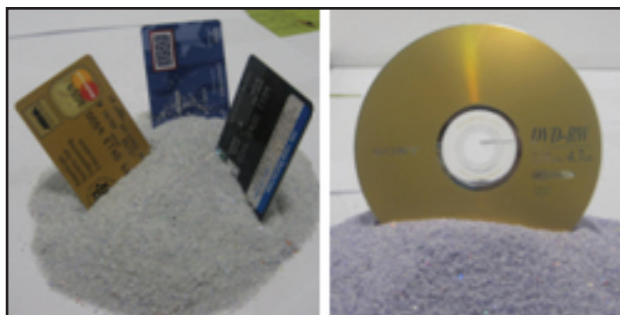
Optical media and plastic cards are crushed into an environmentally friendly powder.
