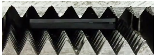
Patented crushing jaws pierce both sides of SSD media
