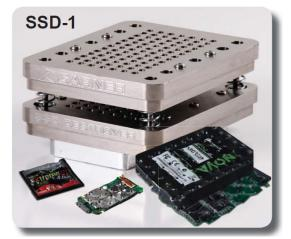
The PD-5 / SSD-1 combination sanitizes solid state media such as SSD, Flash, Compact Flash, USB drives and controller boards for hybrid HDD's. Over 90 pins pierce the solid state media from top and bottom causing both perforation and waffling which destroy the individual memory chips.
