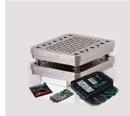
The PD-5 / SSD-1 combination sanitizes solid state media such as SSD, Flash, Compact Flash, USB drives and controller boards for hybrid HDD's. Over 90 pins pierce the solid state media from top and bottom causing both perforation and waffling which destroy the individual memory chips.
